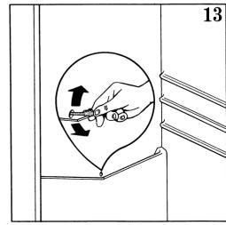
The freezer compartment will become progressively covered with frost. This frost acts as an insulator and thus prevents the cold from reaching the food, this should be removed whenever the frost exceeds 5 mm (1/4 inch).
